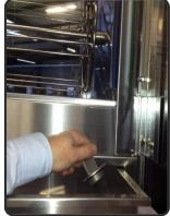
**5.2** - Drain water from the pan cleaning
