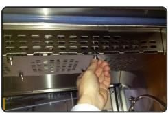
**5.3** - Once a week: remove the stainless steel protection in the ceiling to clean it. (Unscrew the 4 nuts "butterfly")
