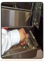
**2.** Drain cooking grease pan with a bucket
