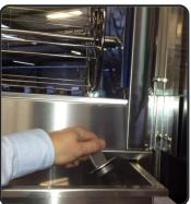
**7.1** After the cycle, drain the water from the pan and place a wet cloth inside the enclosure to complete the cleanup.
