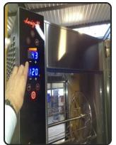
1. Before you begin, the rotisserie must be empty with a temperature below 50°C (shown on the display)
