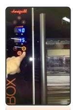
4. Close the door and press the "clean" button to start the program (15 min appear)
